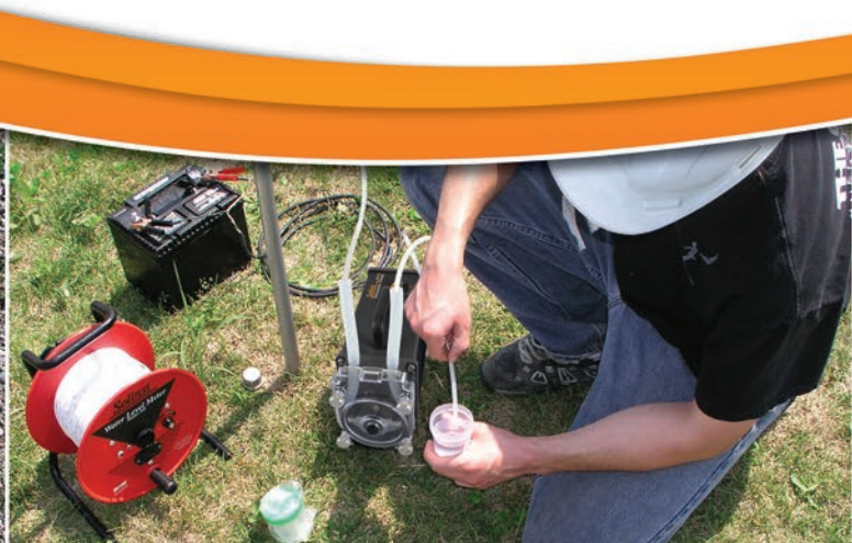
The Drive-Point Profiler provides depth discrete data across a site.
